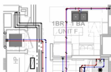
configurations, confusion is common as plumbers quickly move from one configuration to the next, causing a decrease in installation quality and an increase in installation time. To manage this challenge, Uponor Kitting Services includes a blueprint layout of the unit in each bag, so the installer knows exactly where the pipe needs to go and where to make the connections.
